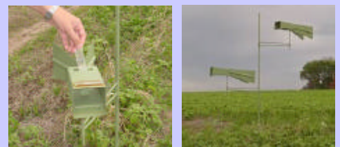
Fig. 2. Spore trap. Inside the weather-vane box, the urediniospores are collected in a slide placed at 45°. (Photos by J.C. Velázquez, INTA EEA Paraná).
